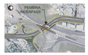
This option will use tunnels to get pedestrians and cyclists under the rail lines. The tunnels would be behind the existing bridge piers. Tunnels generally suffer from a "stranger danger" as it is harder to design them with open sight lines that provide for outside observation. We have been told that there is no possibility of an AT pathway over Pembina if this option is chosen.
