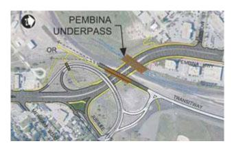
This option will replace the existing bridge, but will move the new bridge further north to widen the gap between the Pembina Underpass and Jubilee Overpass. This will necessitate the relocation of the rail lines, as was done as part of the first stage development of the SWRTC. This is the option being recommended by Bike to the Future.
